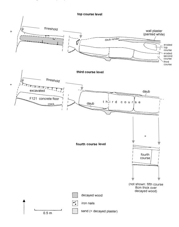
Fig 16 Detail of Period 4 clay-block wall F118.
