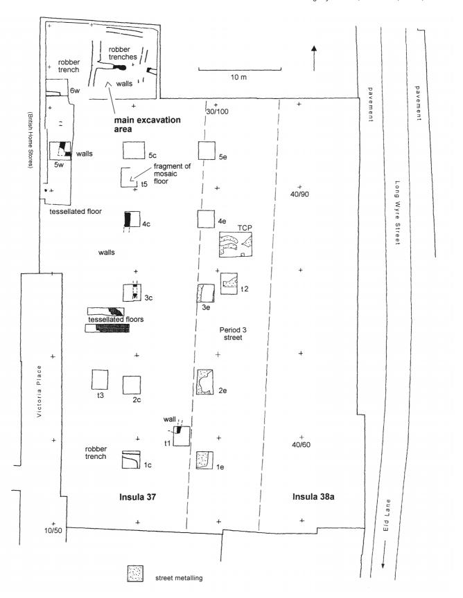
Fig 9 Roman foundations, tessellated floors, robbed walls and street dividing Insulas 37 and 38a. Also showing 1997 evaluation trenches (t1-t3, t5), 1998 pile caps and tower crane pit (eg 1c, 5w, and TCP). Pile cap 6c and T4 are omitted from the plan in order to show the wall lines clearly.
