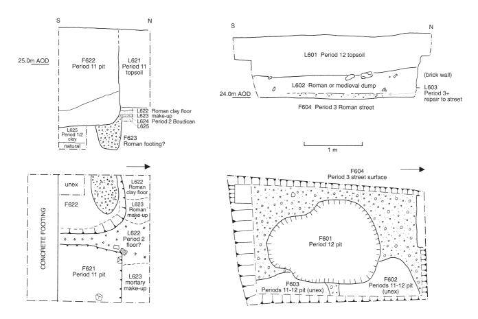
Fig 27 Pile-caps 2 centre (left) and 2 east (right): plan and section.
