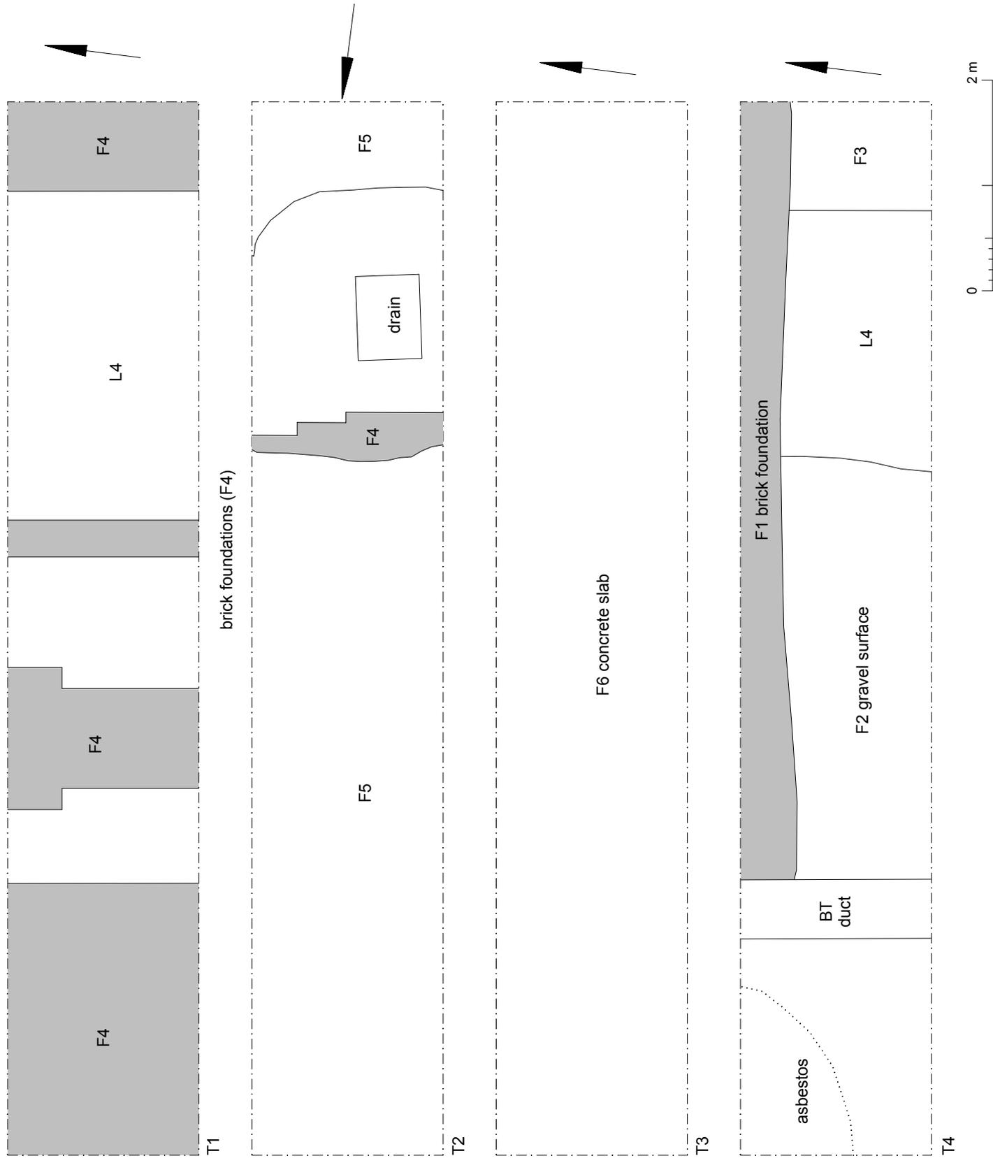
Fig 2 T1-T4: plans (foundations toned grey).
