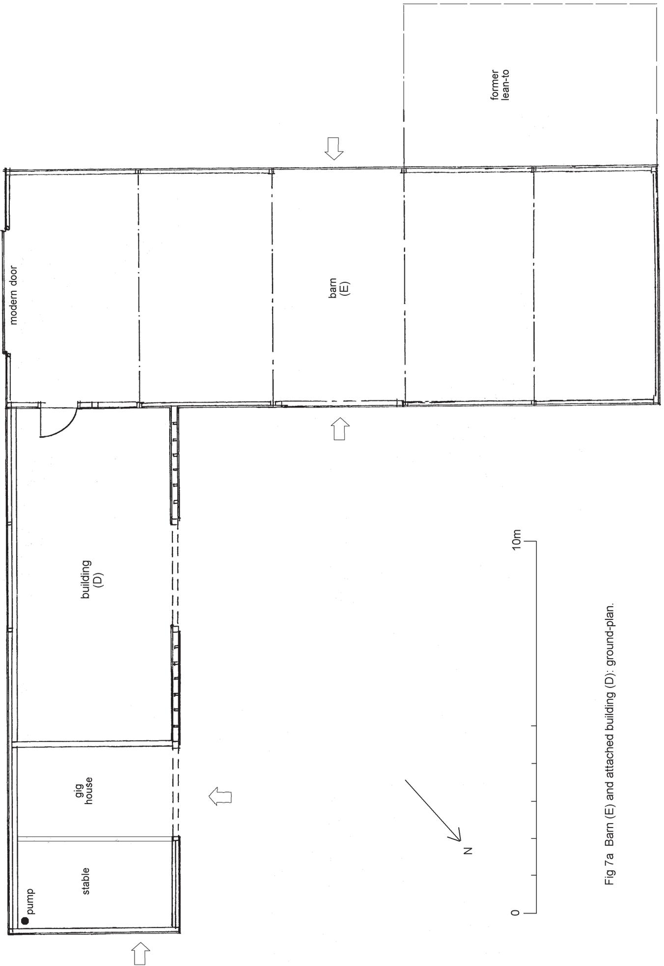
Fig 7a Barn (E) and attached building (D): ground-plan.
