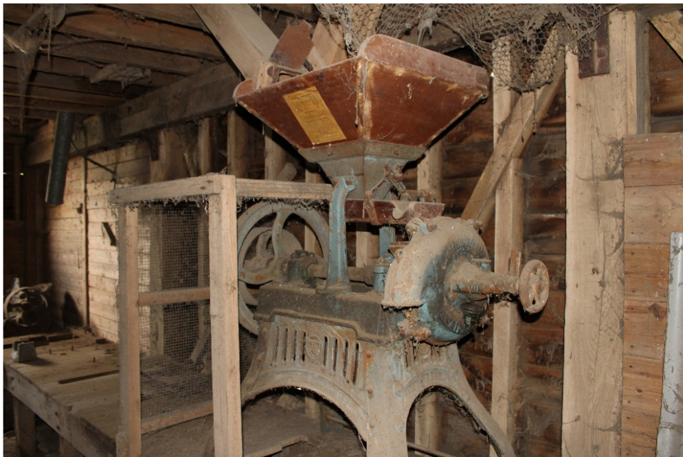
Plate 10 Victorian belt-driven grinder by Bamfords on the first floor of the mezzanine. The slots for the transfer belts can be seen in the top of the workbench and the oil cake breaker can be seen on the far left - view west
