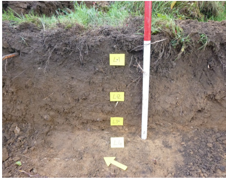
Plate 1 Representative trench section showing soil layers (L1-3) and natural (L4)
