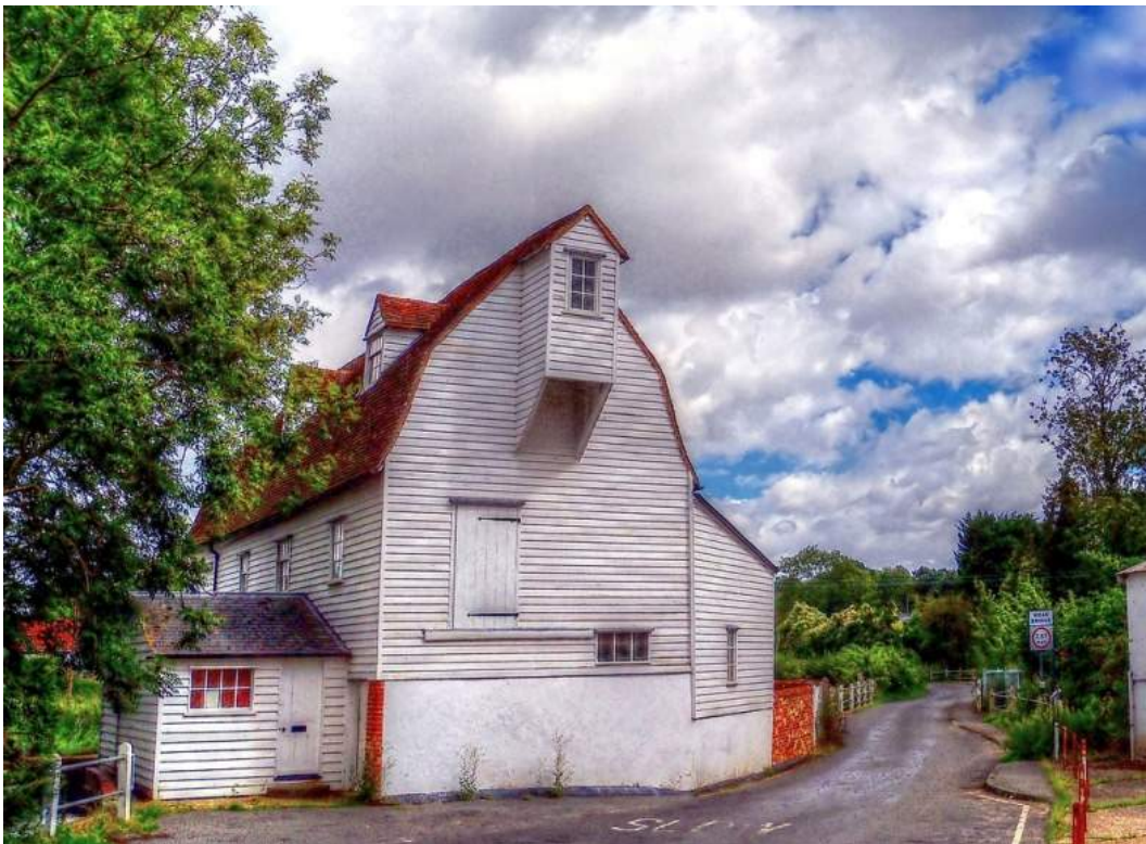
Photograph 24 Alderford Water Mill, Sible Hedingham shares many characteristics with Cannock Mill, including a weatherboarded timber frame, an outward-opening loading door on the first floor, small sash windows and a lucam (Photograph by Bruce Hatton).
