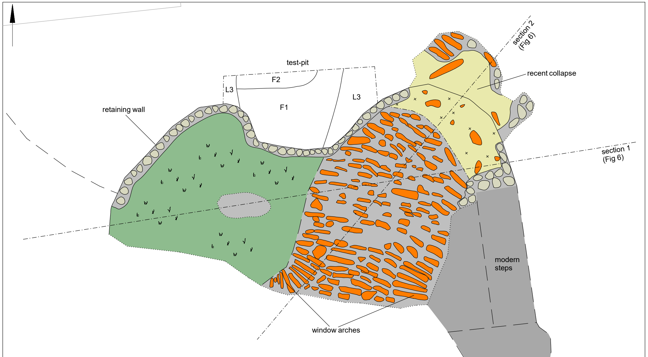
Fig 3 Detailed plan of collapsed masonry and test pit.
