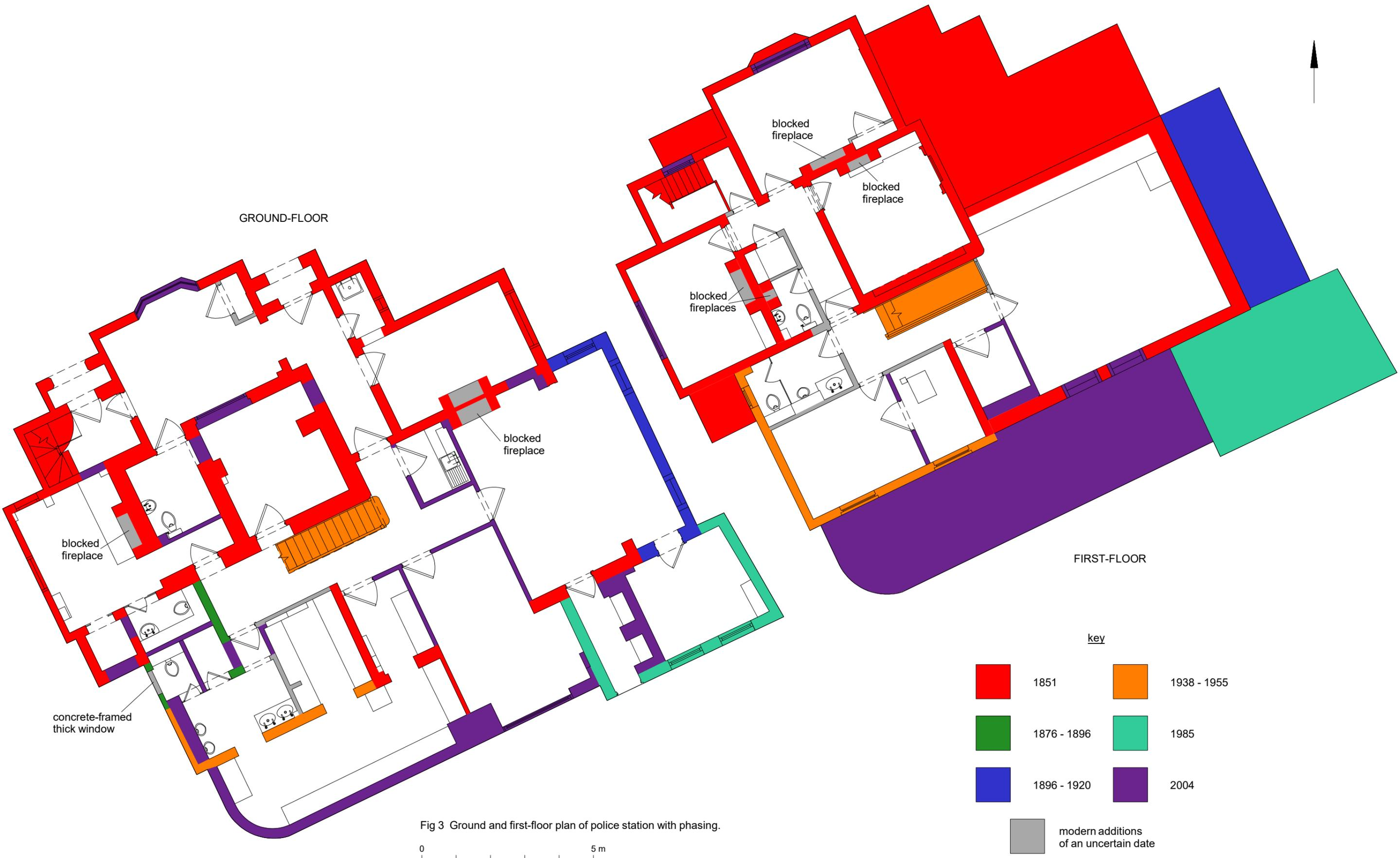
Fig 3 Ground and first-floor plan of police station with phasing.
