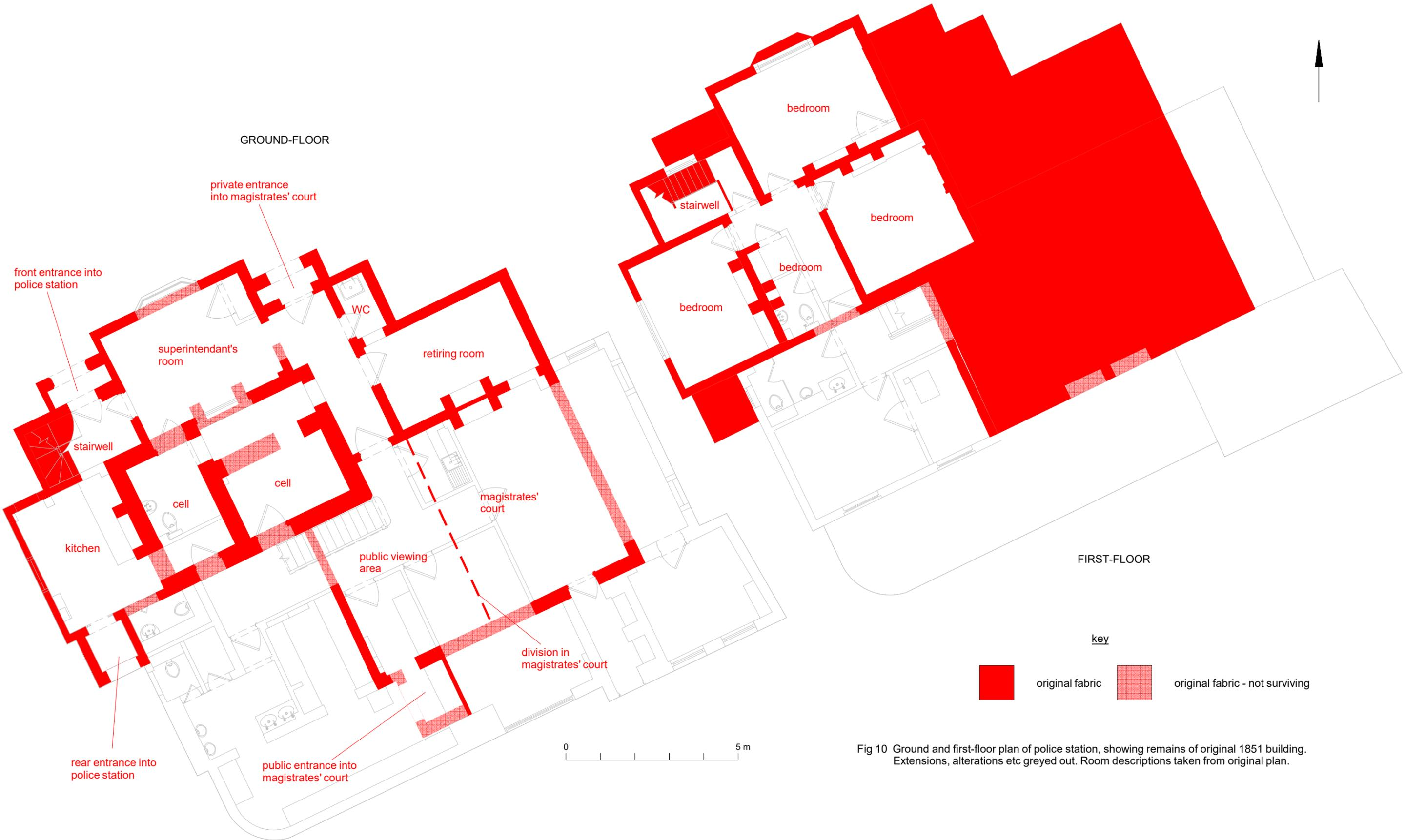
Fig 10 Ground and first-floor plan of police station, showing remains of original 1851 building. Extensions, alterations etc greyed out. Room descriptions taken from original plan.
