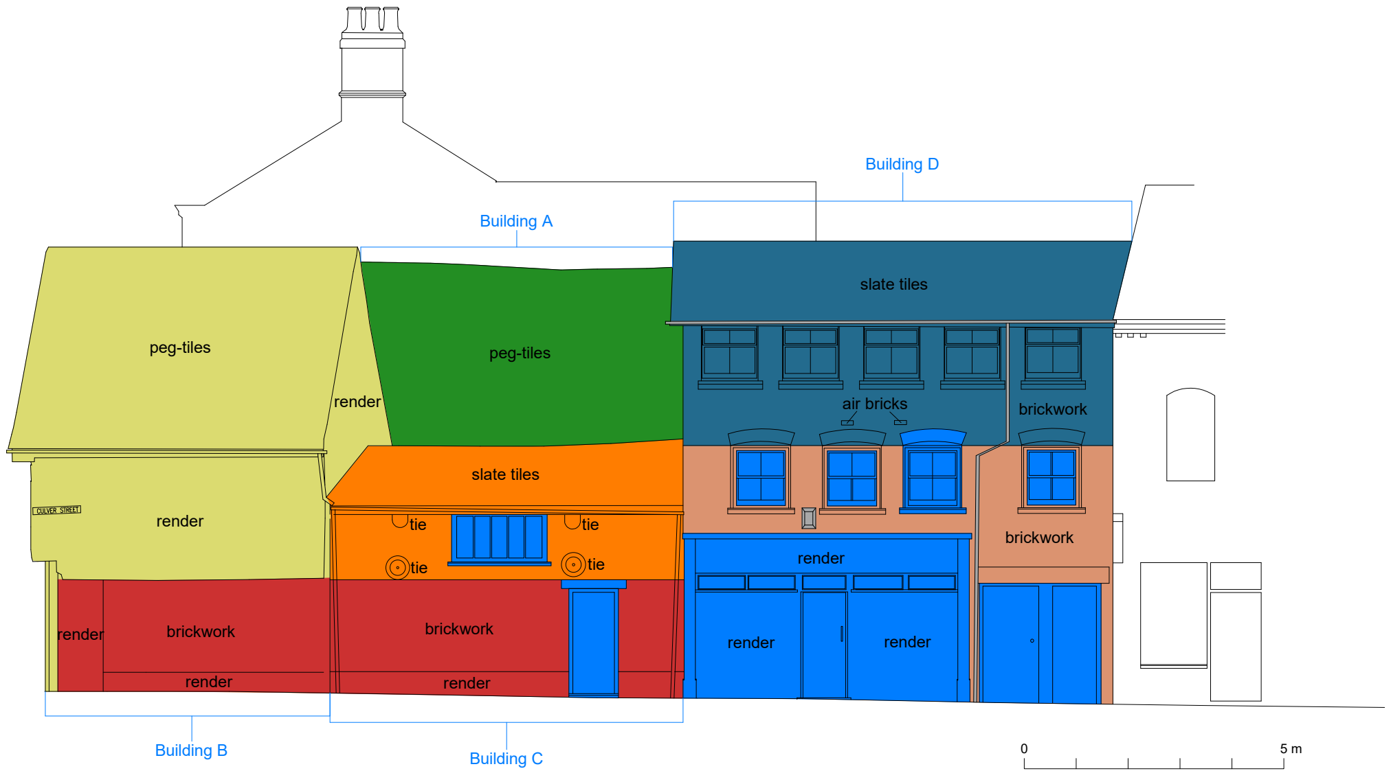
Fig 7 Southern elevation of buildings with phasing.
