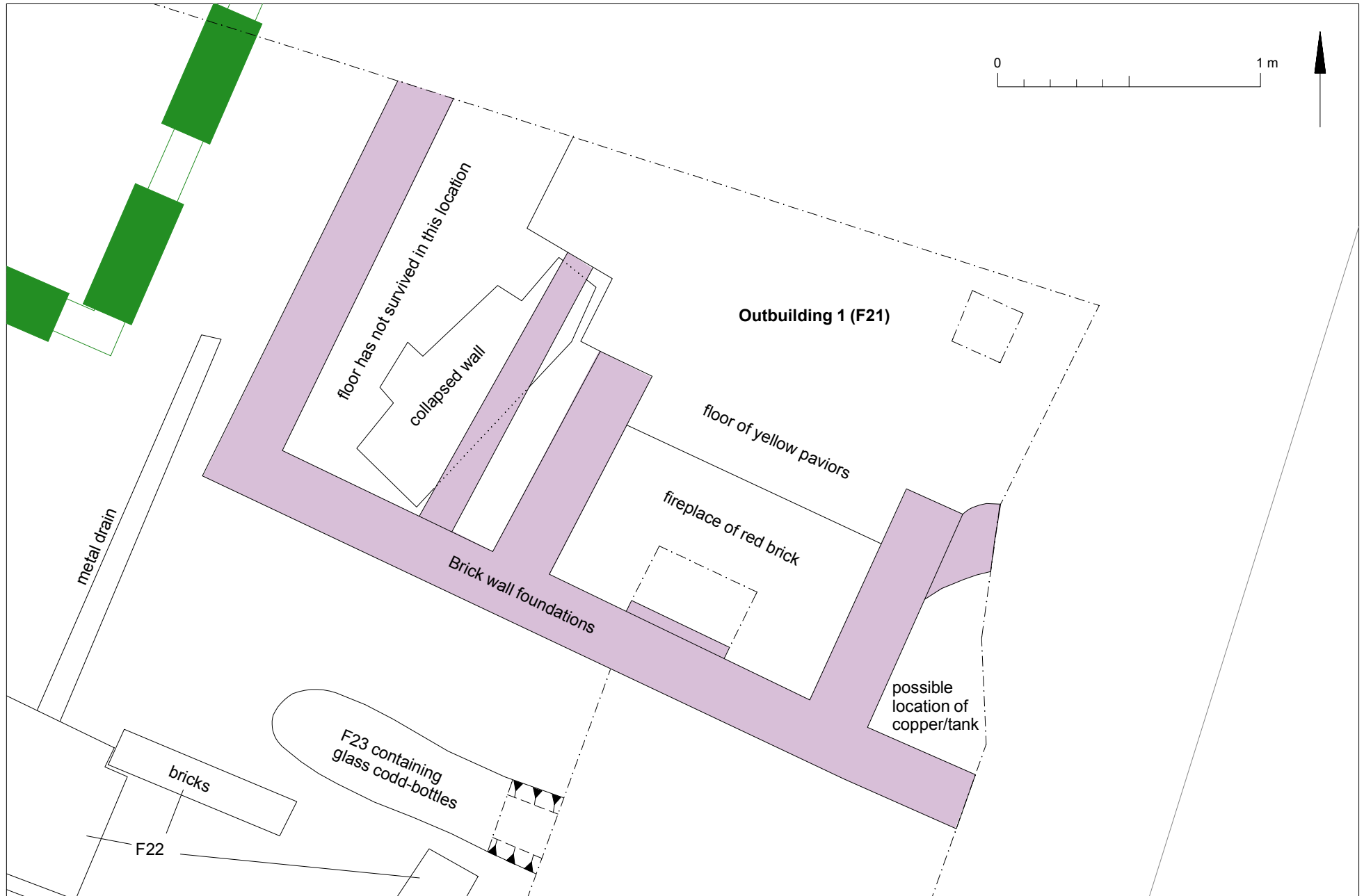
Fig 4 Close-up of Outbuilding 1 (F21)
