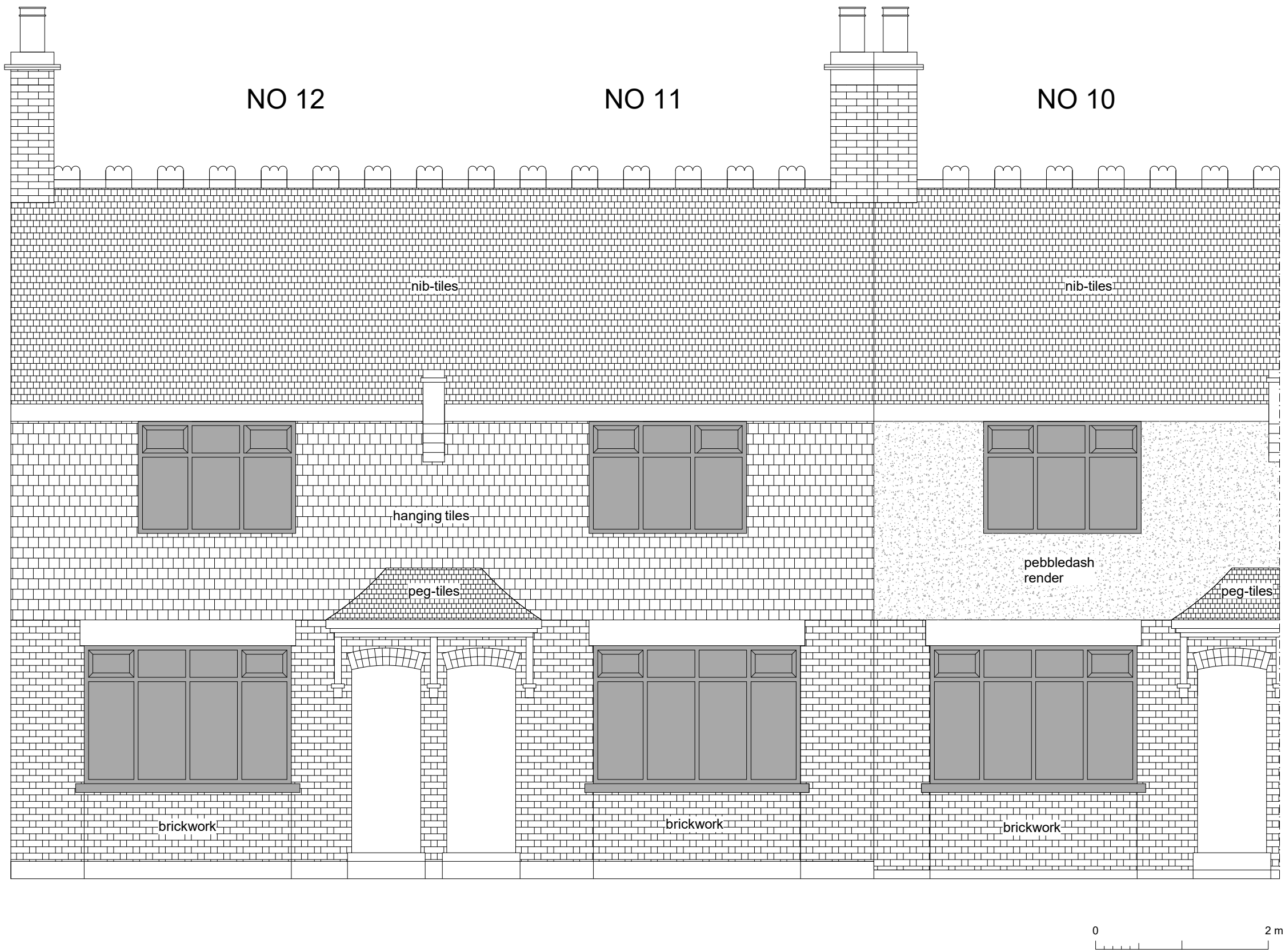
Fig 4 North-east elevation of 10-12 Botany Cottages.
