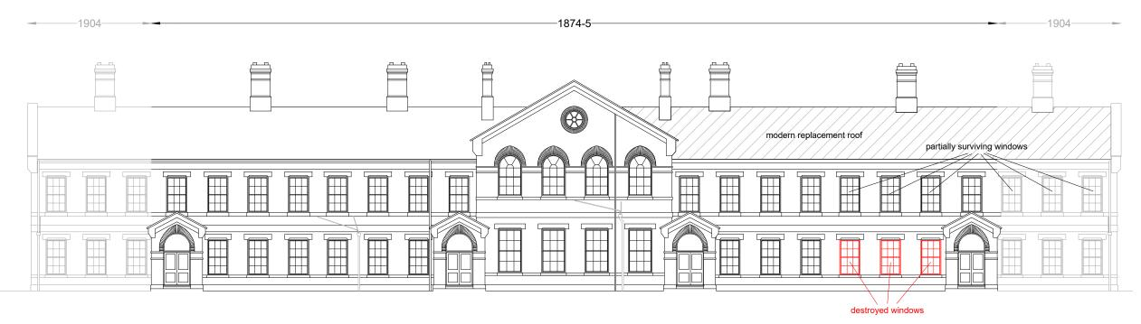
Fig 9 South-east elevation of the former Officers' Quarters, with alterations shown grey.
