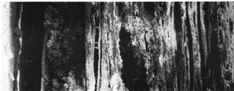
A section through the coats of lime wash on the Roman wall as seen through an electron microscope. The surface of the stone is on the extreme left and the latest coat of white wash is on the extreme right. The section is about 4 mm across.
