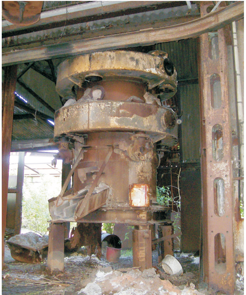
The cupola furnace with the metal-handling monorail at the top of the frame.
